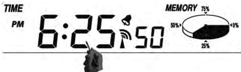
1) Touch the TIME section, + button and – button will be flashing. Touch the + button or – button to adjust the contrast level from 0 to 8. (default 5)
