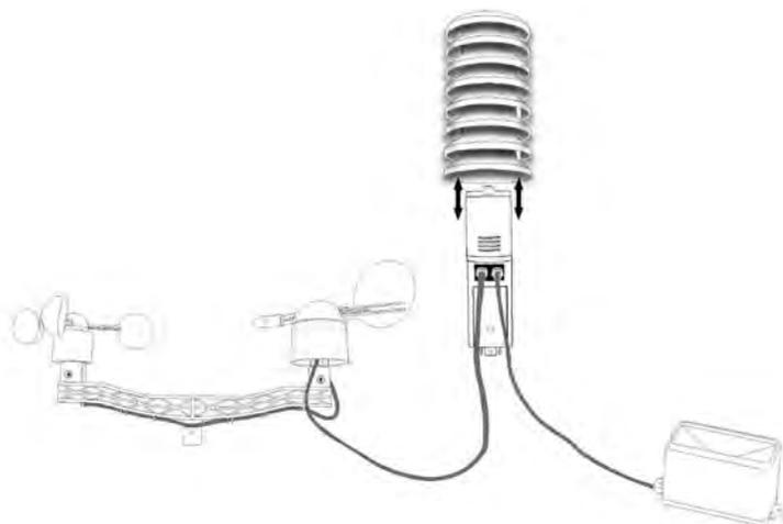
The rain sensor's cable is connected to the input marked Rain on the thermo-hygosensor(see fig.7)
